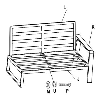
**STEP 6:** Attach Back Rest 3 (L) to the Seat Frame 2 (J) using the M6x45 Bolt (P), Lock washer (U) and Washer (M)
