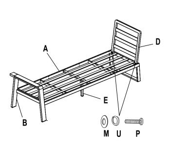
**STEP 2:** Attach Back Rest 2 (D) to the Seat Frame 1 (A) using the M6x45 Bolt (P), Lock washer (U) and Washer (M)
