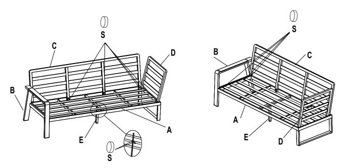
**STEP 4:** Tighten all the bolts on the rightside sofa and cover with the Plastic bolt cap (S). Turn the sofa over.
