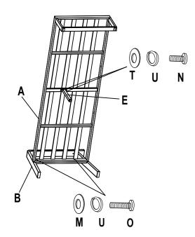
**STEP 1:** Attach Armrest 1 (B) to the Seat Frame 1 (A) using the M6x35 Bolt (c), Lock washer (U) and Washer (M).
