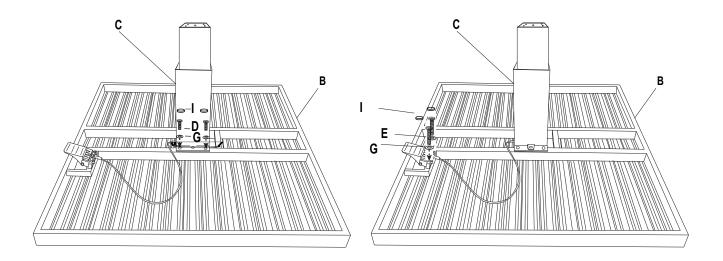
**STEP 1:** Attach Gas pump (C) to the Table top (B), using the M6x25 Bolt (D) and Washer (G). Tighten all the bolts with Allen (K),and cover with the Plastic bolt cap (I).
