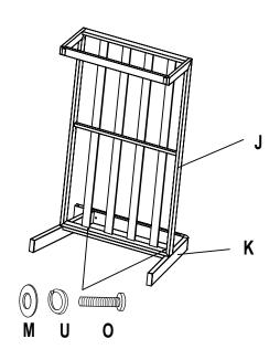
**STEP 5:** Attach Armrest 2 (K) to the Seat Frame 2 (J) using the M6x35 Bolt (O) ,Lock washer (U) and Washer (M)
