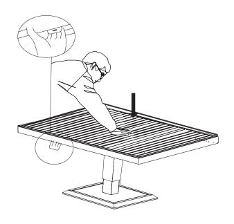
**STEP 5:** Press down in the center of Table top while squeezing the handle to lower the table top
