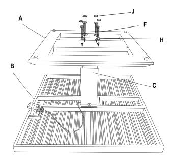
**STEP 3:** Attach Base (A) to the the Gas pump(C), using the M8x50 Bolt (F) and Washer (H). Tighten all the bolts with Allen (K), and cover with the Plastic bolt cap (J).
