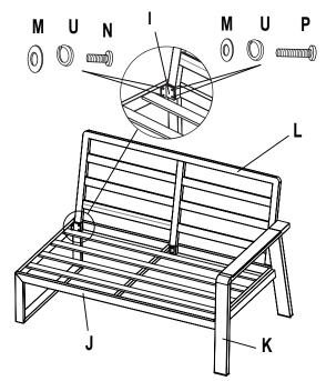
**STEP 8:** Attach the Connector Bracket (I) to Back Rest 3 (L), on one side using the M6x45 Bolt (P), Lock washer (U) and Washer (M). Secure on the other side of the Connector Bracket using the M6x20 Bolt (N), Lock washer (U) and Washer (M)
