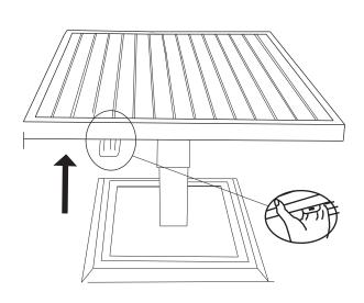
**STEP 4:** Turn the Table over. Squeeze the handle to raise the table top
