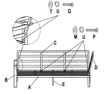
**STEP 3:** Attach Back board 1 (E) to Seat Frame1 (A) using the M6x45 Bolt (d), Lock washer (U) and Washer (M). Attach Back Rest 1 (C) to the Armrest 1 (B)
