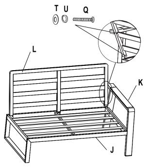
**STEP 7:** Attach Back Rest 3 (L) to the Armrest 2 (K) using the M6x55 Bolt (Q), Lock washer (U) and Washer (T)
